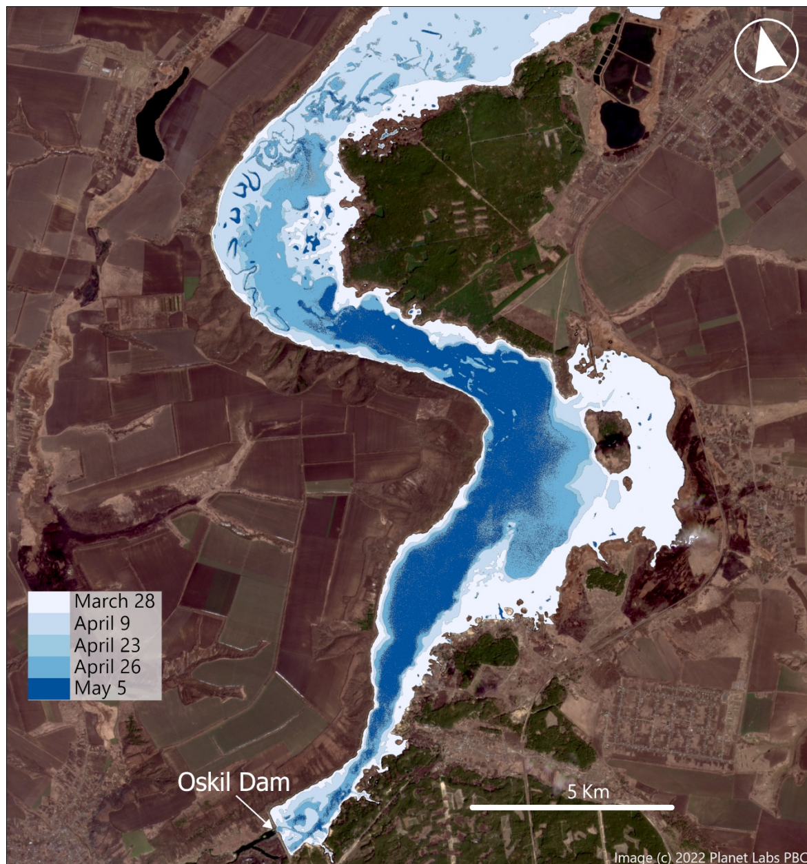
Figure 4: Water masks for the first five dates (March 28–May 5, 2022) in time-series analysis demonstrate changes in reservoir water levels following damage to the dam in late March 2022.
